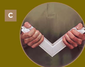
C Pinch fusion-welding
